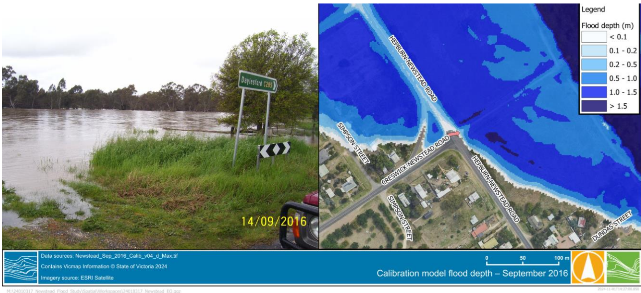
Figure 4-12 Creswick-Newstead Rd/Hepburn-Newstead Rd intersection, captured at around 1400 hours on 14 September 2016. Agrees well with modelled peak flood extent.
